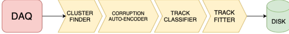
Figure 5: The CLAS12 raw data is passed through four neural networks with the last one outputting the full parameters of the tracks (momentum and direction), which can be used for the identification of the event topology and and physics analysis.
