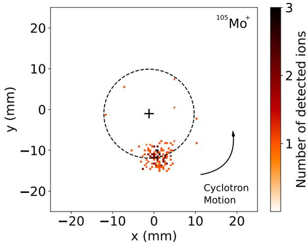
Figure 3. Projection of the cyclotron motion of  $^{105}\text{Mo}$  ions onto the position-sensitive detector obtained with the PI-ICR technique using a phase accumulation time  $t_{\text{acc}} = 500$  ms. The average excitation radius is indicated with the dashed circle and the position of the center spot with the + symbol. Only one state is present.
