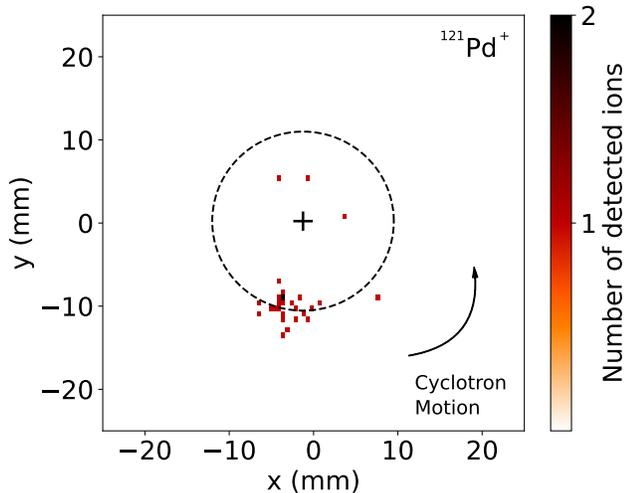
Figure 5. Projection of the cyclotron motion of  $^{121}\text{Pd}$  ions onto the position-sensitive detector obtained with the PI-ICR technique using a phase accumulation time  $t_{\text{acc}} = 329$  ms. The average excitation radius is indicated with the dashed circle and the position of the center spot with the + symbol.
