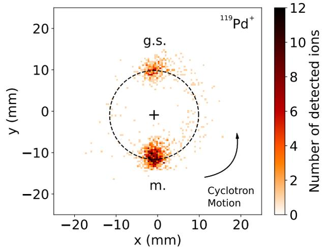
Figure 4. Projection of the cyclotron motion of  $^{119}\text{Pd}$  ions onto the position-sensitive detector obtained with the PI-ICR technique using a phase accumulation time  $t_{\text{acc}} = 284$  ms. The average excitation radius is indicated with the dashed circle and the position of the center spot with the + symbol.
