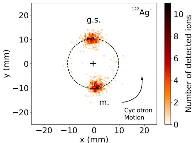
Figure 7. Projection of the cyclotron motion of  $^{122}\text{Ag}^+$  ions onto the position-sensitive detector obtained with the PI-ICR technique using a phase accumulation time  $t_{\text{acc}} = 200$  ms. The average excitation radius is indicated with the dashed circle and the position of the center spot with the + symbol.
