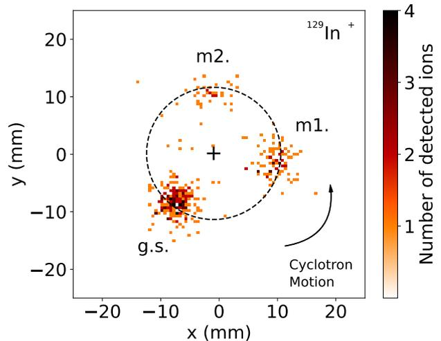
Figure 1. Projection of the cyclotron motion of  $^{129}\text{In}$  ions onto the position-sensitive detector obtained with the PI-ICR technique using a phase accumulation time  $t_{\text{acc}} = 208$  ms. The average excitation radius is indicated with the dashed circle and the position of the center spot with the + symbol.
