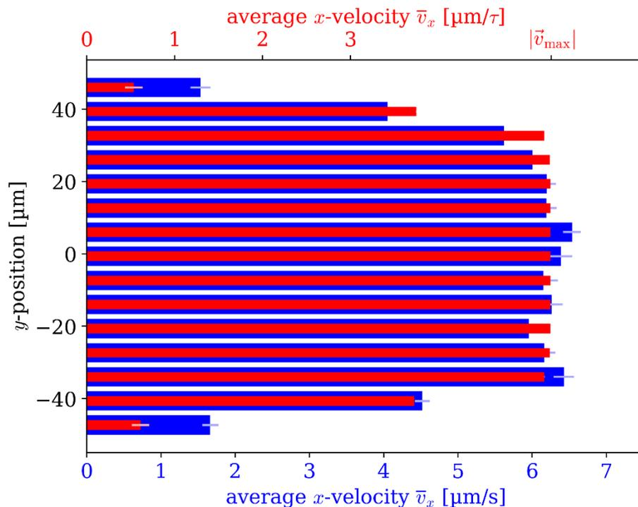
**Figure 2:** Skyrmion flow velocity profiles of the modulated channel of 80  $\mu\text{m}$  width. Comparison of experimental (blue) and simulated (red) velocity profiles. Both profiles become flat in the inner part of the channel.
