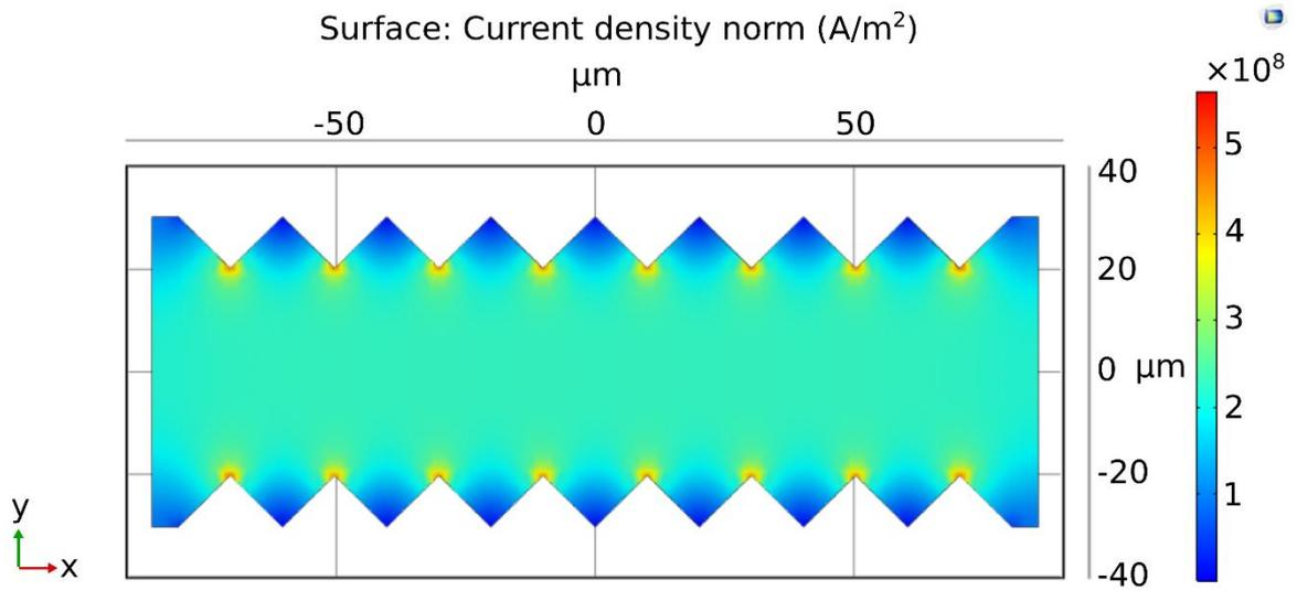
**Supplementary Figure 2:** COMSOL simulation of the current distribution in a 40 $\mu\text{m}$  wide modulated channel. The current density in the middle section of the channel can be considered constant, while it becomes highest at the inward-pointing spikes.
