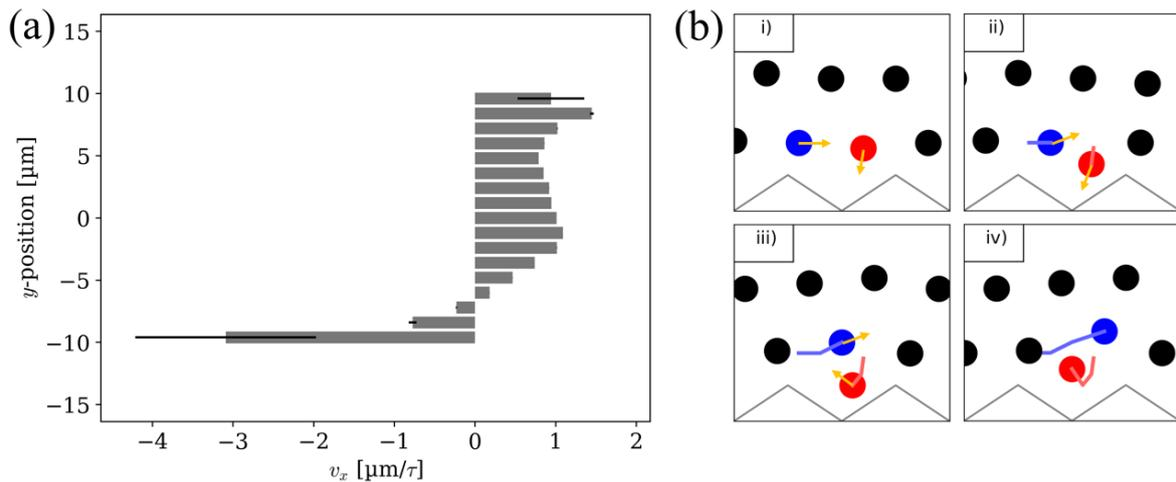
**Figure 3:** a) Simulated velocity flow profile of a 20  $\mu\text{m}$  channel with oblate modulation (see b)) and a skyrmion Hall angle set to  $\theta_{skHA} = 15^\circ$ , resulting in an asymmetric velocity flow profile. Notably, the average skyrmion velocity at the lower edge of the confining geometry is negative, implying that skyrmions in this region flow opposite to the applied driving force. b) Sketch of a dynamic process
