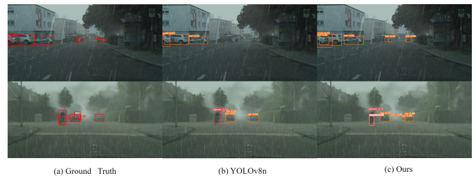
Fig. 6. Detection results of our proposed method. (a) Ground truth, (b) Baseline(Yolov8s), (c) our D-YOLO. As we can see, our D-YOLO generates more bounding box with higher confidence score.
