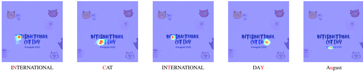
Figure 8. Visualization of the cross attention maps within our Glyph-SDXL model. We show the heat maps between all pixels and the selected characters from the text box with ‘INTERNATIONAL CAT DAY’ and ‘8 August 2022’.
