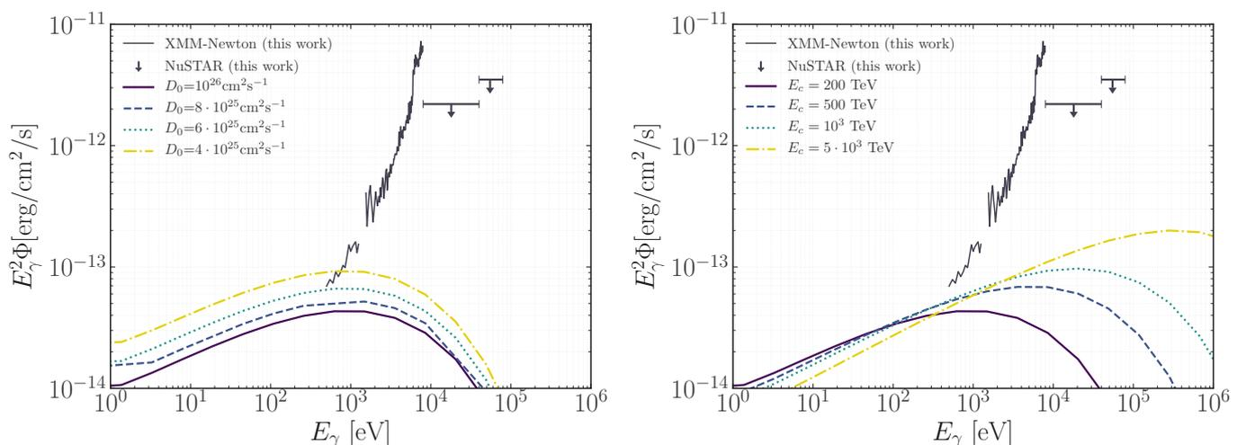
**Fig. 9.** The synchrotron emission from the Geminga pulsar halo as compared to the upper limits in the X-ray band obtained in this work using *XMM-Newton* and *NuSTAR* data when varying the diffusion coefficient  $D_0$  (left panel) and the energy cutoff of the electron source term (right panel). See text for details.
