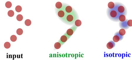
**Fig. 1.** The input is indicated by the red dots. The green ellipses indicate the **anisotropic** Gaussian kernels while the blue circles indicate the **isotropic** Gaussian kernels. Although anisotropic Gaussian is more representative in terms of geometry, it leads to the computation difficulties. In contrast, isotropic Gaussian is more computational efficient.
