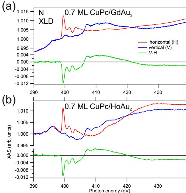
FIG. S1. XLD at the N L<sub>2,3</sub> edge at RT on (a) CuPc/GdAu<sub>2</sub> and (b) CuPc/HoAu<sub>2</sub> samples. Spectra were recorded with both, vertical (in red) and horizontal (in blue) polarized light at a fixed incident angle of 70°. The green one is the difference between the signals measured with horizontal and vertical polarized light.
