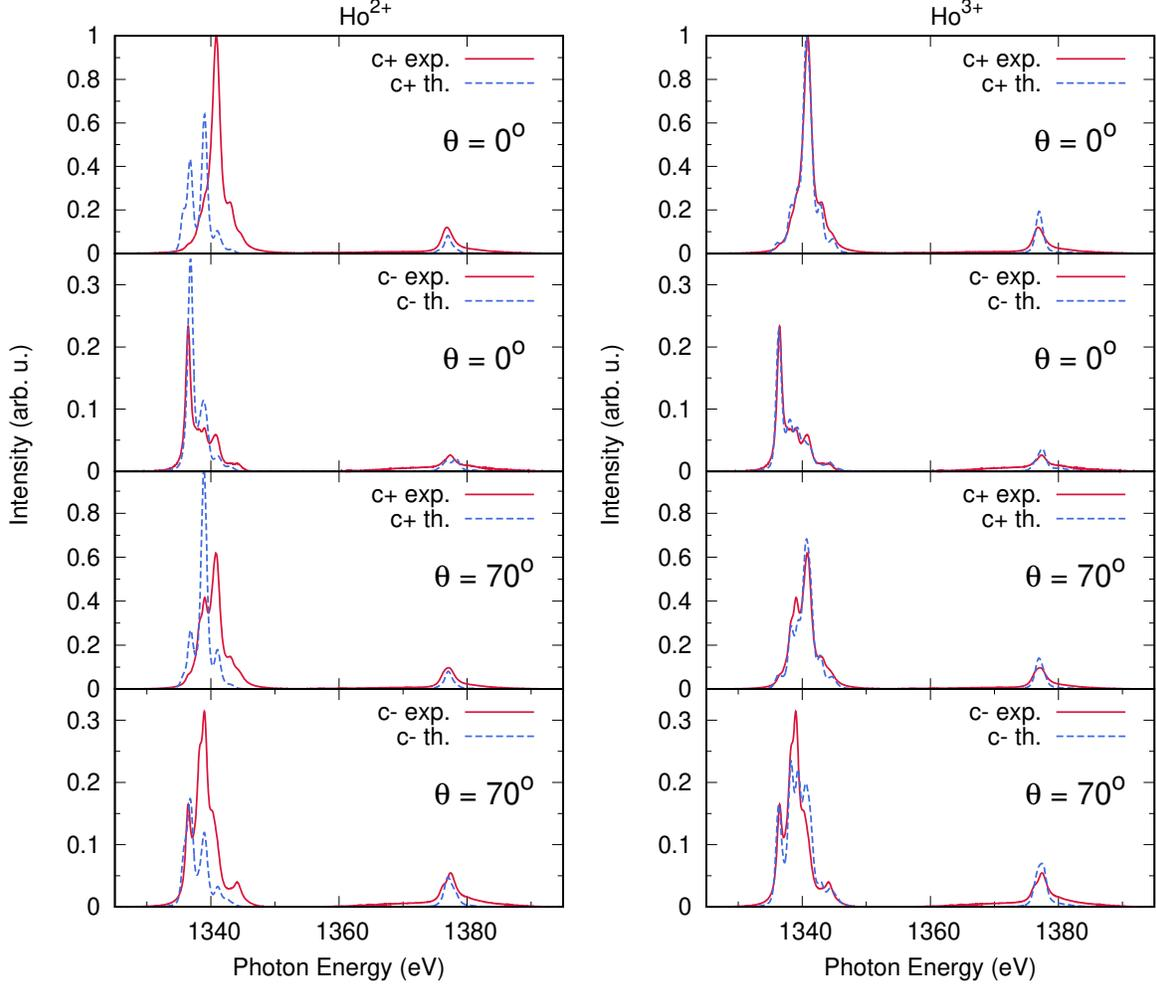
FIG. S3. Set of four X-ray absorption spectra (both circular light polarizations and both external magnetic field directions). Solid and dashed curves represent, respectively, the experimental data and the theoretical simulation assuming  $\text{Ho}^{2+}$  (left) and  $\text{Ho}^{3+}$  (right) valence states.
