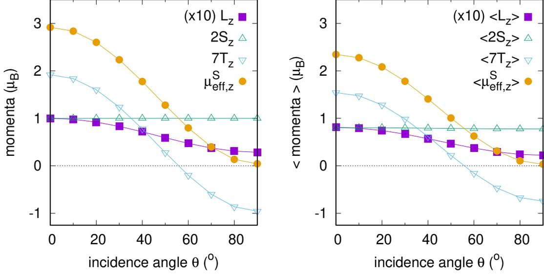
FIG. S5. Projected  $L_z$  (values scaled by a factor 10),  $2S_z$ ,  $7T_z$  and  $\mu_{eff}^{S,z} = 2S_z + 7T_z$  momenta on the applied field direction for the bare CuPc molecule, using the orbital energies of Ref. [13]. Left:  $T = 0$  K saturation values. Right: expectation values at  $\mu_0 H = 6$  T and  $T = 4$  K.
