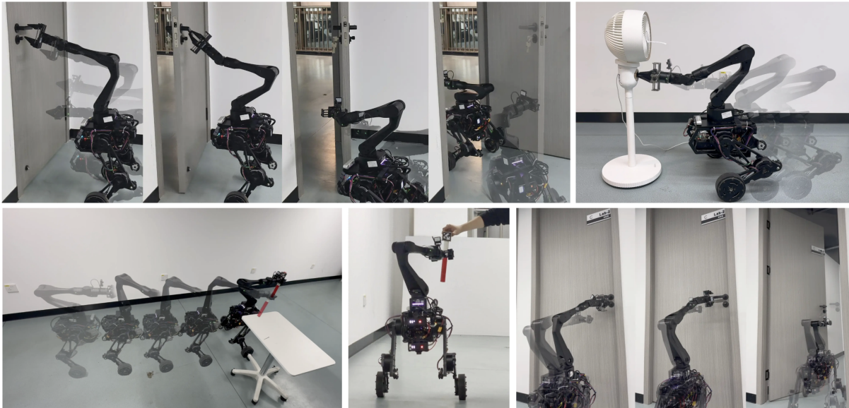
Fig. 1. Tasks accomplished by the proposed architecture. Top-Left: door-opening-and-pulling task; Top-Right: fan-knob-twitching task; Bottom-Left: relay-baton-chasing task; Bottom-Right: door-opening-and-pushing task.
