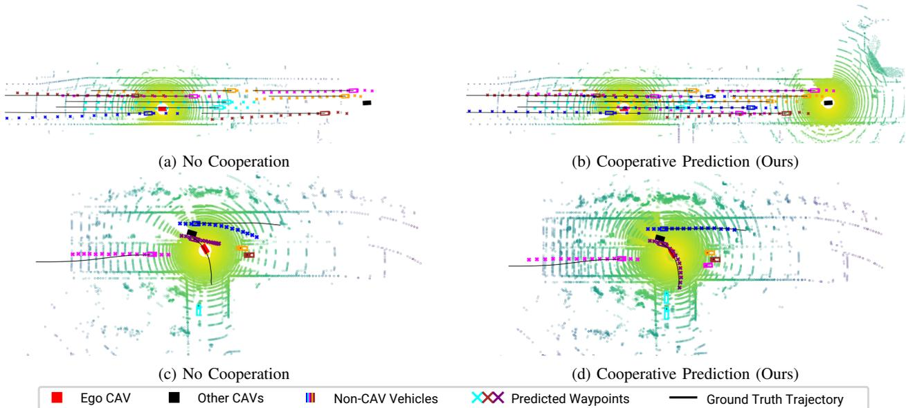
Fig. 3: The visualizations of predicted trajectories under different model settings in two traffic scenarios. In (a) and (c), some surrounding vehicles are not detected and the predicted trajectories (colored waypoints) without cooperation deviate significantly from the ground truth (black lines). In contrast, in (b) and (d) where cooperative prediction is enabled, the predicted trajectories become closer to the ground truth due to additional useful information from others.
