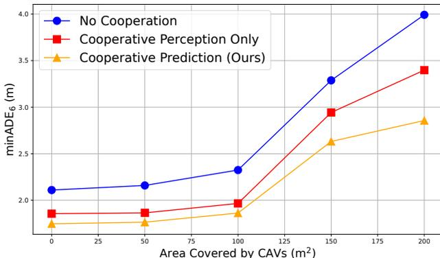
Fig. 4: A comparison of motion prediction performance at 5s prediction horizon under different areas covered by CAVs in OPV2V. The area is calculated based on the smallest convex hull that covers all the CAVs. As the number of CAVs increases in different scenarios, more areas are likely covered, which boosts the performance gap between no cooperation and cooperative prediction.
