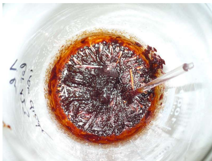
Figure 1.: Heat treated and cooled down the shiny, dry mass of reaction product of iron nitrate and oleic acid.
