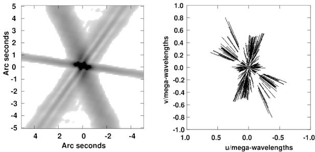
**Figure 1.** Right:  $uv$  plane coverage for a typical snapshot observation with the hybrid A/AnB configuration used during the 2020 observations, at declination  $+20^\circ\text{N}$ . Left: point-spread function (dirty beam) resulting from this  $uv$  coverage.
