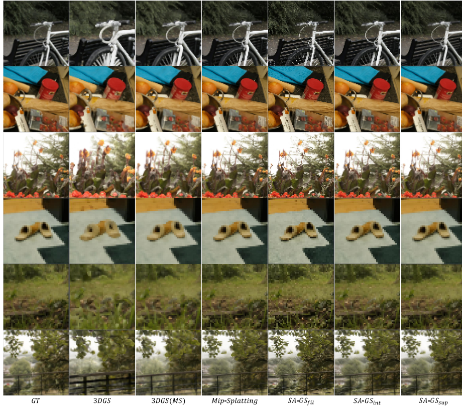
Fig. 6: Single-scale Training and Multi-scale Testing on the Mip-NeRF 360 Dataset. All methods are trained on full resolution ( 1\times ) and evaluated on smallest resolution ( 1/8\times ) to mimic zoom-out case. Our 2D scale-adaptive filter maintains the consistency of the Gaussian across different rendering settings. SA-GS_{int} achieves results comparable to Mip-Splatting, while SA-GS_{sup} surpasses Mip-Splatting, resulting in optimal performance for this setting.
