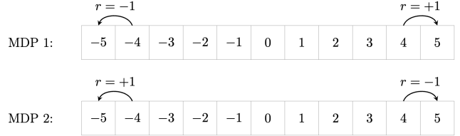
Figure 2: Two GridWorld MDPs. Their initial states are 0. In MDP 1 (top), transiting from state 4 to 5 generates a reward of +1 and transiting from state -4 to -5 yields a reward of -1 . In MDP 2 (bottom), the signs of the rewards are flipped.
