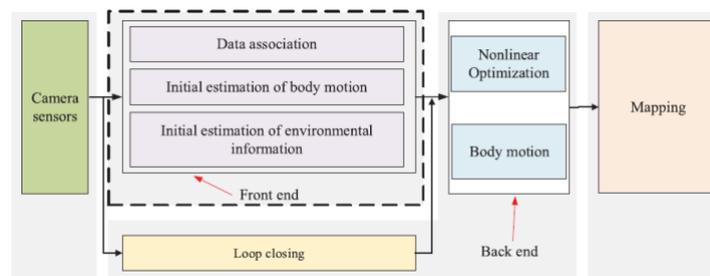
**Figure 1.** Visual SLAM system architecture diagram
