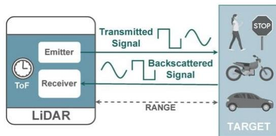
**Figure 3.** How LiDAR works
