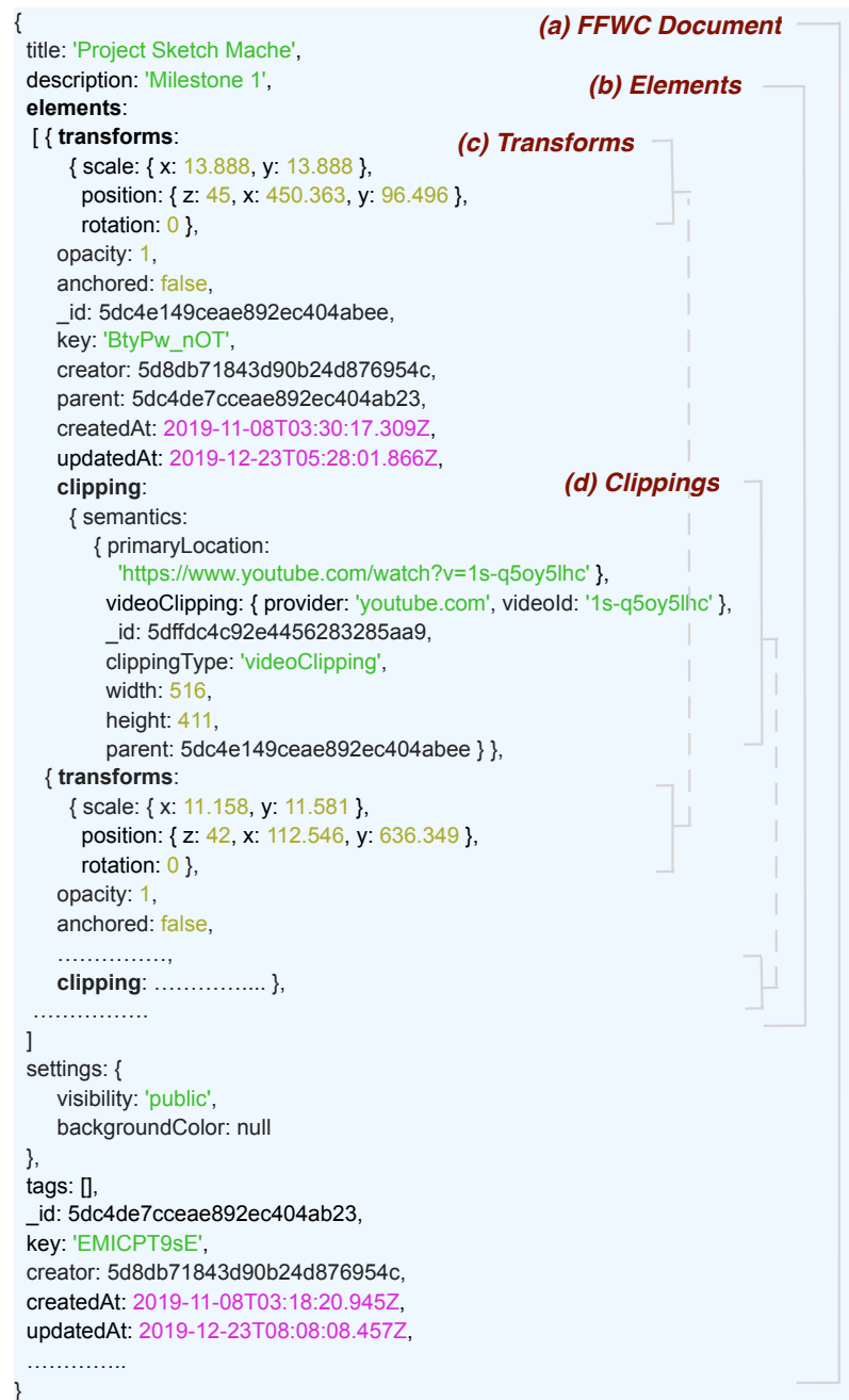
Fig. 2. Each multiscale design document—a free-form web curation (FFWC)—is stored as JSON [40]. It is comprised of properties such as title , description , creator , and a collection of elements . Each element includes a transforms property—with sub-properties position , scale , and rotation —which allows determining the element’s spatial location with respect to the origin. Each element also stores a clipping property, which in turn stores semantics extracted at the time of collecting the element.
