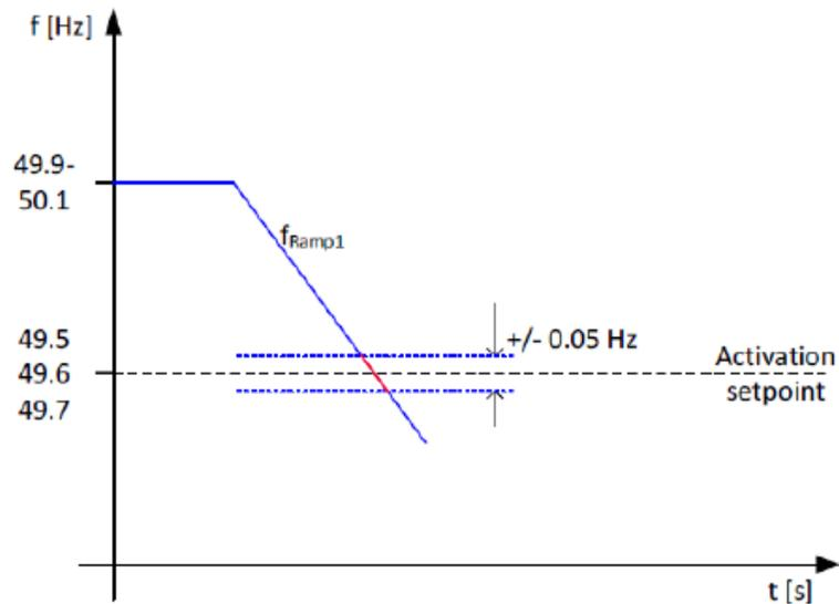
Figure 5 Ramp test for FFR compliance verification.
