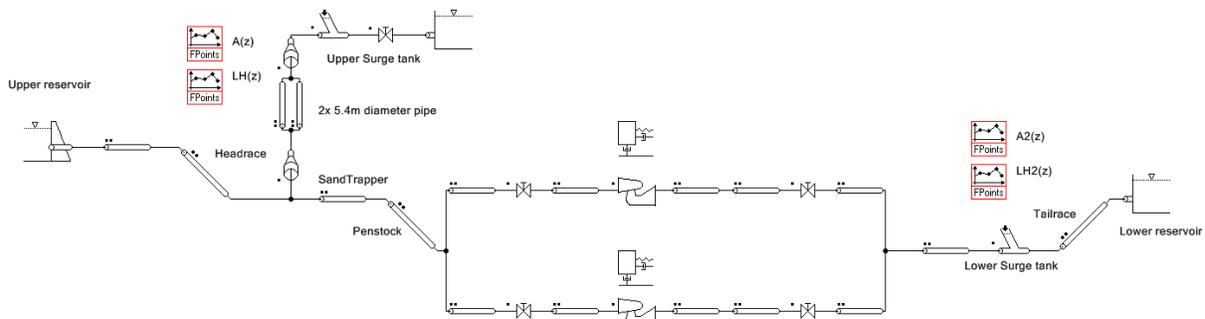
Figure 8 1D SIMSEN simulation model of the 2 x 395 MW Frades 2 pumped storage power plant.
