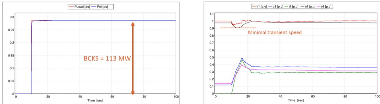
Figure 13 Variable speed - BCK in turbine mode with initial speed at  $n_{middle}$  - Output power response (left) and corresponding transient behaviour of unit 1 (right). (right graphs with  $h$ : net head,  $q$ : discharge,  $t$ : torque,  $n$ : rotational speed,  $y$ : guide vane opening of unit 1).
