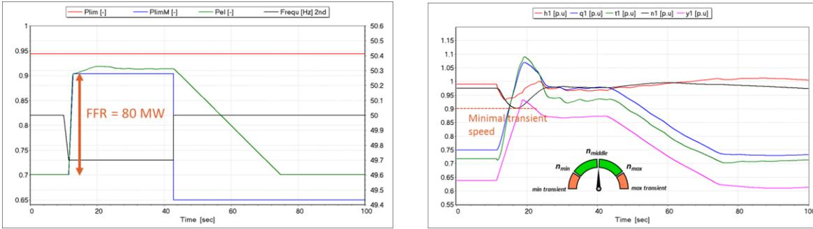
Figure 12 FFR in turbine mode with initial speed at  $n_{middle}$ . Output power response (left) and corresponding unit transient behavior (right). (right graphs with  $h$ : net head,  $q$ : discharge,  $t$ : torque,  $n$ : rotational speed,  $y$ : guide vane opening of unit 1).
