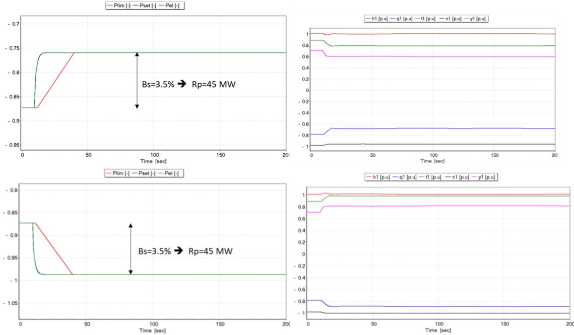
Figure 10 FCR in pump mode - Output power response (left) and corresponding unit transient behavior (right) to a frequency deviation of  $\pm 200\text{mHz}$  with  $B_s=3.5\%$  and  $n_{ini}=n_{middle}$ . (right graphs with  $h$ : net head,  $q$ : discharge,  $t$ : torque,  $n$ : rotational speed,  $y$ : guide vane opening of unit 1).
