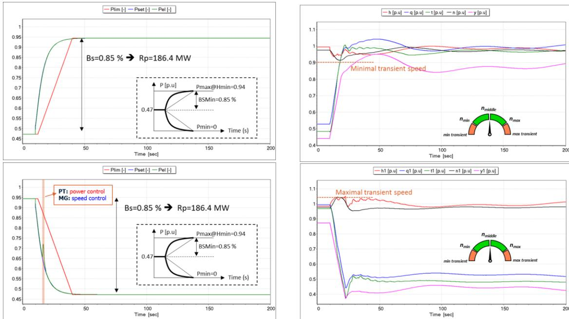
Figure 9 FCR in turbine mode - Output power response (left) and corresponding unit transient behavior (right) to a frequency deviation of  $\pm 200\text{mHz}$  with  $B_s=0.85\%$  and  $n_{ini}=n_{middle}$ . (right graphs with  $h$ : net head,  $q$ : discharge,  $t$ : torque,  $n$ : rotational speed,  $y$ : guide vane opening of unit 1).
