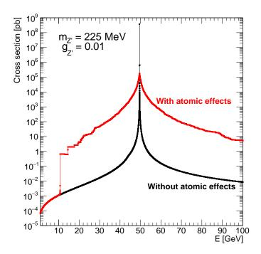
**Figure 3**. Total atomic cross section for the process  $e^+e^- \to Z' \to \nu\bar{\nu}$  on lead as a function of the impinging positron energy, considering (red) or not (black) the motion of atomic electrons.
