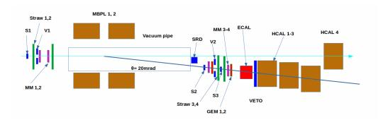
Figure 1. Schematic representation of the NA64-e detector, searching for an invisibly decaying Z' produced by the interaction of 100 GeV electrons with the material of the active ECAL target. See text for further details.
