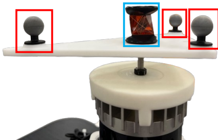
Figure 5. Sensor placement for the IMU-Prism calibration. Reflective balls for motion capture cameras (MCC) and the prism are marked in red and blue, respectively. We use MCC’s measurements to infer high-rate motion of the prism.
