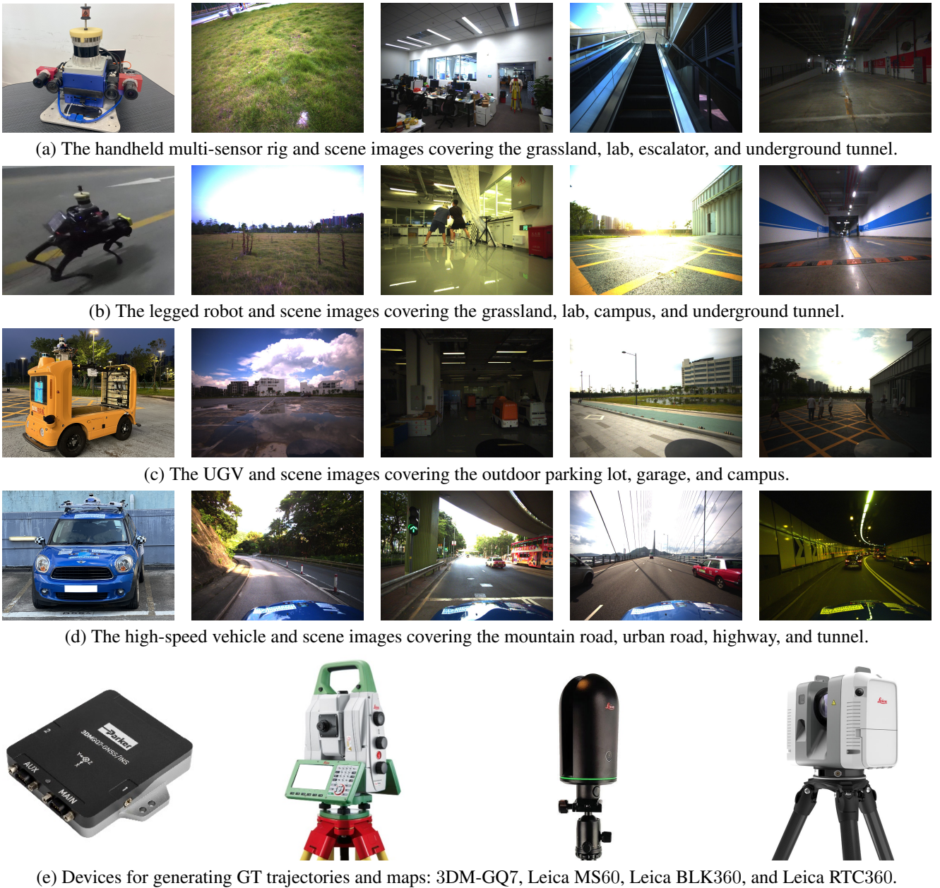
Figure 4. Platform-Specific Data Samples: (a) The handheld multi-sensor rig across various environments, (b) the legged robot, (c) the low-speed UGV, (d) the high-speed vehicle, and (e) the GT generation device. The depicted scenes highlight the FusionPortableV2 dataset’s comprehensive coverage across a spectrum of platforms and environmental conditions.
