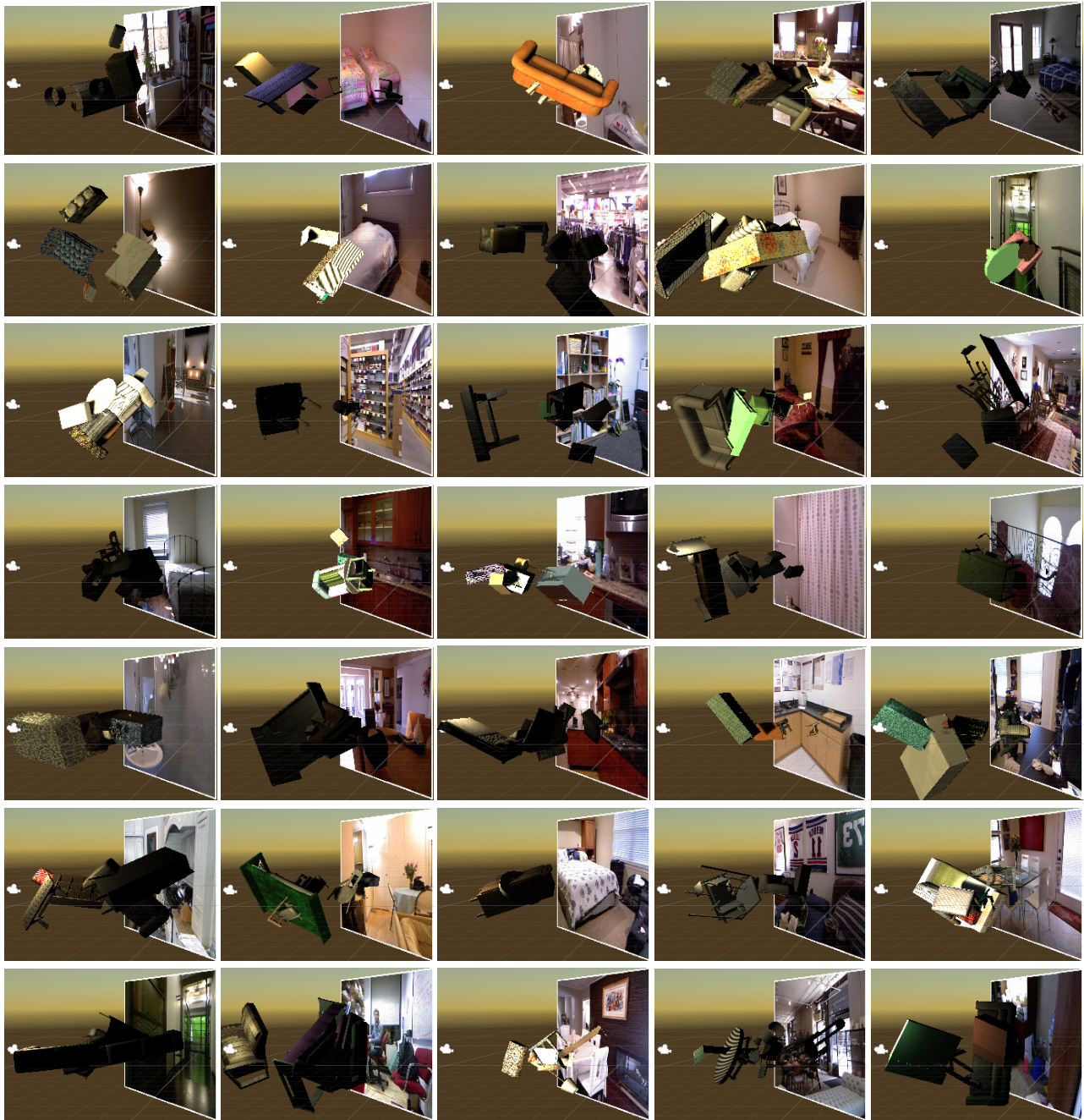
Figure 10. Screenshots of the Unity 3D at the initial stage of image virtualization: the distance between the virtual camera (left) and the NYU-v2 image plane (right) determines how many virtual objects can be effectively placed between the camera and the image plane.
