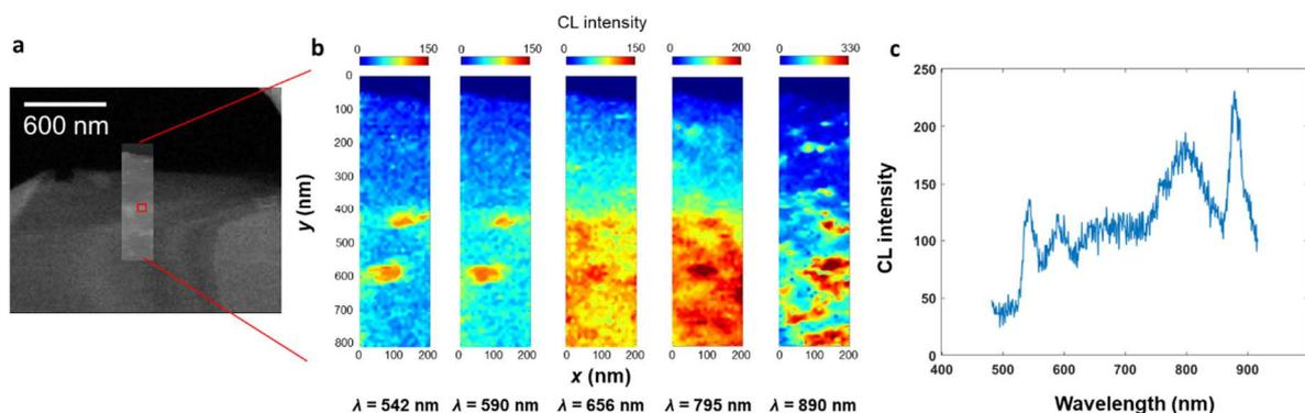
**Figure S6: Position of different atomic defects.** (a) SEM image of the hBN flake on the holey carbon support film. (b) Spectral images shown at depicted wavelengths. (c) CL spectrum at the position marked by the red box on the SEM image.
