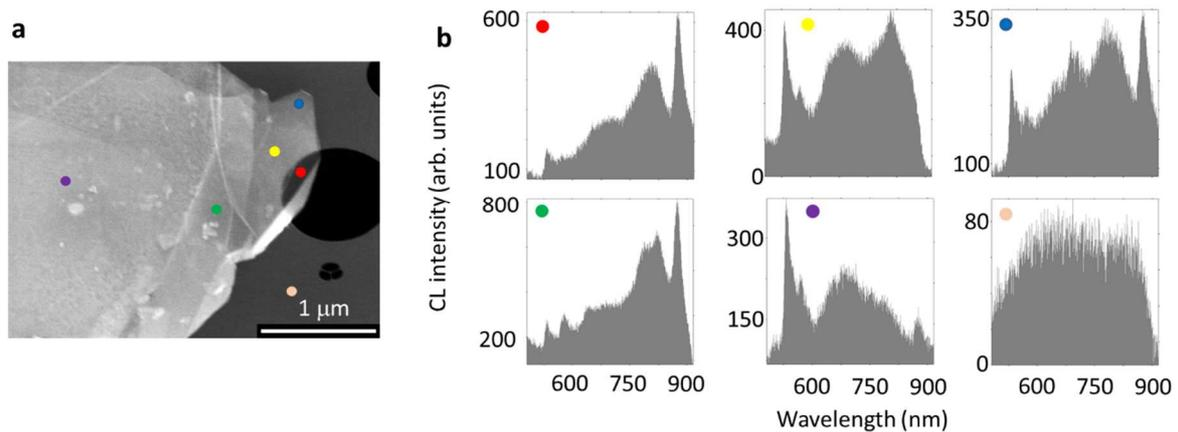
**Figure S5: Excitation of different atomic defects with electron beams.** SEM image of the hBN flake on the holey carbon support film. Each colored point represents a unique impact position of the electron beam. The resulting CL spectra are shown on the right, revealing the individual emission pattern for each excitation spot. The spectra on the bottom right depict the CL response of the underlying carbon film.
