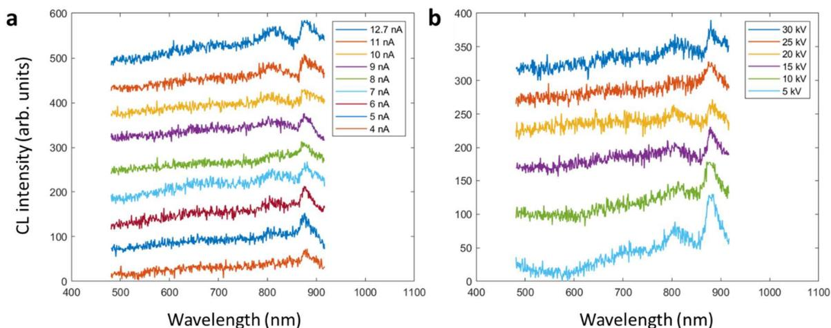
**Figure S8: Changing electron beam characteristics.** CL spectra of the hBN flake displayed in Figure 1 of the main text at different values of (a) beam current and (b) acceleration voltage as indicated in the figure.
