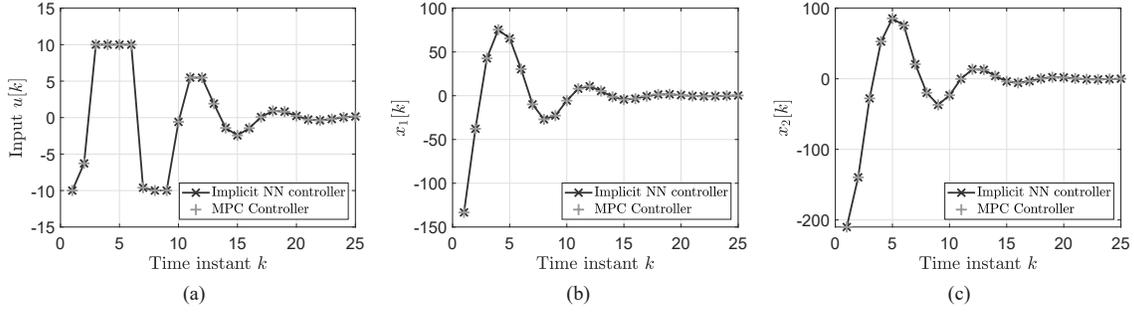
Figure 2: Comparison between the MPC controller and the implicit neural network defined by (11) for the numerical example. The input sequences  $u[k]$ , and states  $x_1[k]$ ,  $x_2[k]$  are shown for both policies. The equivalence between the two simulations validates the results of the paper. Note that the implicit neural network captures the input constraints imposed by the MPC policy, as predicted.
