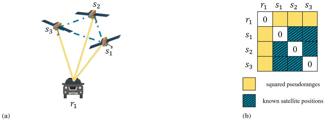
**FIGURE 3** A combination of squared pseudoranges and known satellite positions are used to construct the EDM shown in subfigure (b) for the system shown in subfigure (a) of a single receiver and three satellites. Subfigure (b) taken from Knowles and Gao, 2023b.
