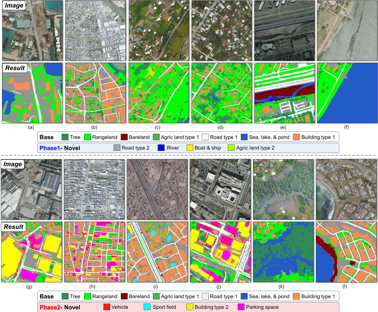
Figure 11. The visual results of final land-cover maps produced by the SegLand. The patches of (a–f) are sampled from the test images of challenge phase 1 . The patches of (g–l) are sampled from the test images of challenge phase 2 .
