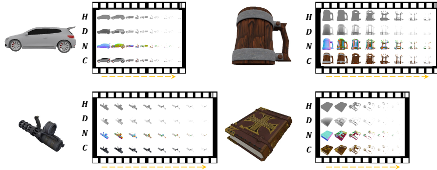
Figure 2: Samples of our X-Ray 3D sequential representation. Given a viewpoint, we capture the 3D attributes multi-layer surface frames, including hit H , depth D , normal N , and color C , in a video format. Noted that the number of frames in an X-Ray varies depending on the complexity of the 3D objects. The dotted yellow lines indicate the ray or sequence direction.
