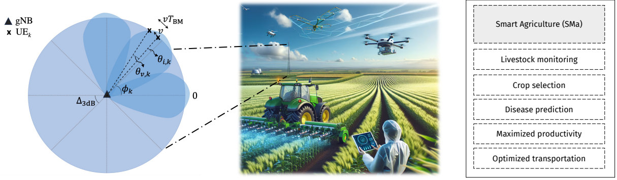
Fig. 1. UE mobility model (left) and SMA scenario (right). During beam management, UE_k accumulates an angular offset \theta_k due to initial misalignment ( \theta_{i,k} ) and mobility ( \theta_{v,k} ).
