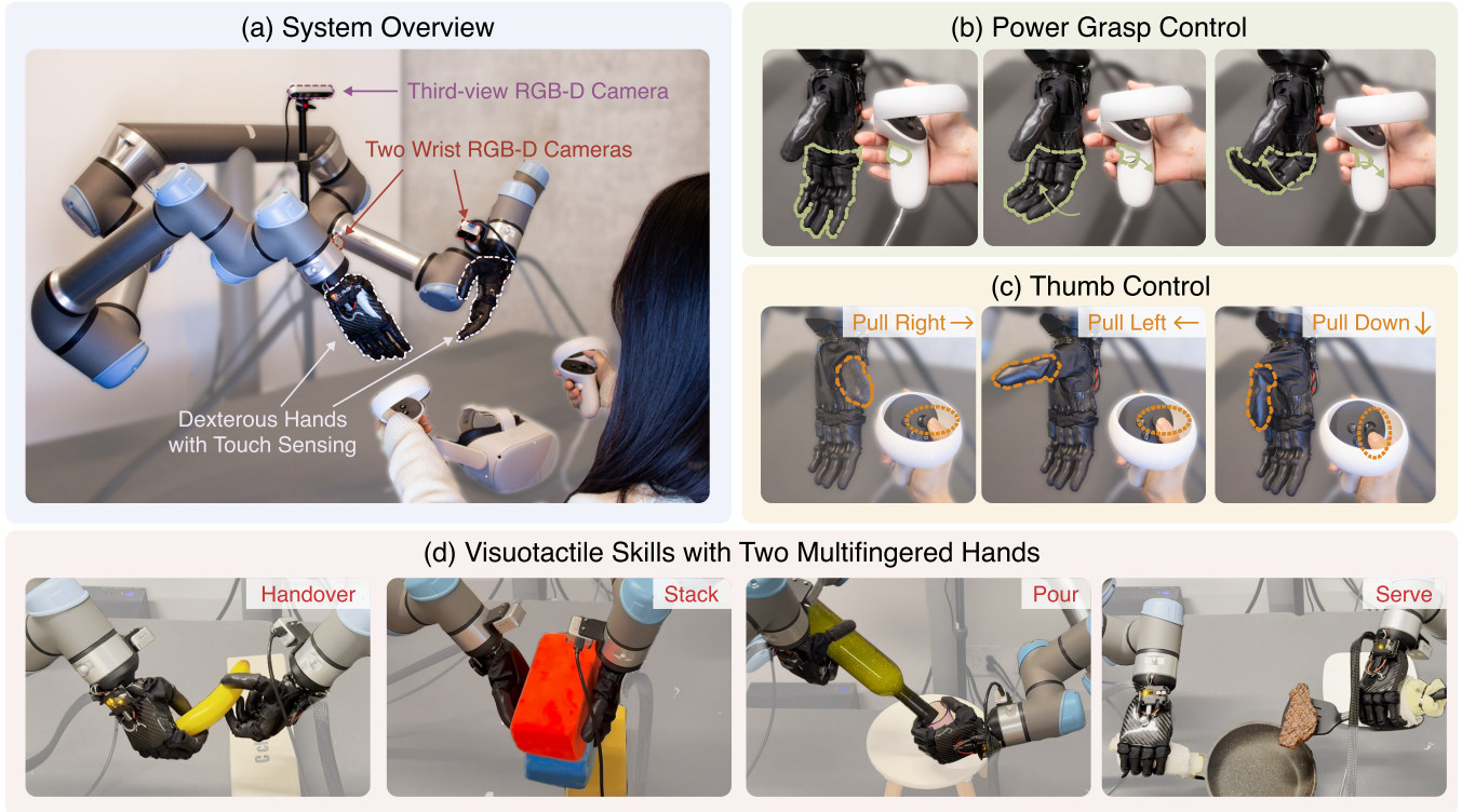
Fig. 1. An overview of our system setup and learned visuotactile skills on four tasks. (a) Our hardware and teleoperation system setup. The hardware consists of two UR5 robot arms, each equipped with a Psyonic Ability Hand. Visual observations are obtained via two wrist-mounted and one third-view RGB-D cameras. Tactile observations come from the multifingered hands, with each fingertip equipped with six touch sensors. We utilize the Meta Quest 2 platform for teleoperation. (b) We use the grip buttons of the Quest controllers to command power grasp of the non-thumb fingers. (c) We use thumbsticks to control the 2-DoF joint positions of the thumbs. (d) Four policies learned from visuotactile data collected by our hands-arms teleoperation system (HATO). These policies can accomplish a variety of complex bimanual tasks: handing over a slippery object, stacking a block tower, pouring from a wine bottle, and serving steak.
