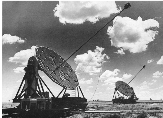
Figure 2: Light collectors used in the Narrabri stellar intensity interferometer. Image from Sky & Telescope, vol. 28, pp. 2-7, 1964.
