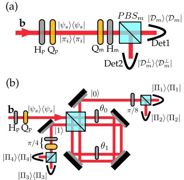
FIG. 6. The proposed experimental setup. (a)  $B^{(1)}(j)$  and  $B^{(2)}(j|i)$  are learned with the data obtained from the detections in Det1 or Det2 after preparing the polarization of the photons in the states  $|\psi_s\rangle\langle\psi_s|$  and  $\Pi_i$ , respectively, using  $H_p$  and  $Q_p$  and projective measurements implemented by  $Q_m$ ,  $H_m$  and  $PBS_m$ . (b)  $B^{(2)}(i)$  learning requires a SIC-POVM measurement, which is performed using the displaced Sagnac interferometer.
