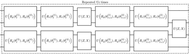
Fig. 1. The fPQC has  $N$  qubits and  $d/2$  layers of parameterized  $U(R_y(\theta_1), R_y(\theta_2))$  and  $U(R_z(\theta_1), R_z(\theta_2))$  gates followed by entangling gates such as  $U(Z, X)$ .
