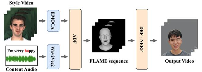
Fig. 1. Overview of ERLNet. EMOCA [6] and Wav2Vec2 [1] are employed for extracting FLAME coefficients and audio features. During the inference process, our approach requires two inputs: a style reference video and a content audio. After passing through the ADF module, a FLAME coefficients sequence matched to the speech is obtained. Subsequently, the DBF-NeRF network takes these FLAME coefficients as input to render the final video.
