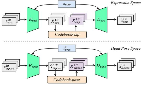
Fig. 2. Structure of FLAME latent space. Expression sequence  $z_{exp}^{1:t}$  and head pose variation sequence  $z_{\Delta pose}^{1:t}$  of length  $t$  are inputs. Two individual VQ-VAEs are used to build the expression space and the head pose space. Emotion vector  $z_{emo}$  and the head pose of the first frame  $z_{pose}^0$  are utilized as conditional inputs. Only decoders and codebooks are frozen and used in subsequent networks.
