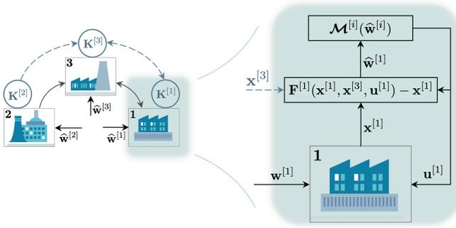
Fig. 3. Example of networked dynamics (33) and decentralized IMC controller for agent  $i = 1$ .
