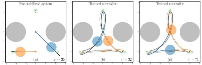
Fig. 7. Waypoint-tracking — Closed-loop trajectories before training (left) and after training (middle and right). Snapshots taken at time-instants  $\tau$ . Colored (gray) lines show the trajectories in  $[0, \tau_i]$  ( $[\tau_i, \infty)$ ). Colored balls (and their radius) represent the agents (and their size for collision avoidance).
