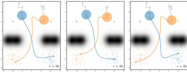
Fig. 9. Mountains — Three different closed-loop trajectories after training a REN controller without  $\mathcal{L}_2$  stability guarantees over 100 randomly sampled initial conditions marked with  $\circ$ . Colored (gray) lines show the trajectories in (after) the training time interval.
