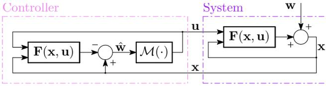
Fig. 1. IMC architecture parametrizing of all stabilizing controllers in terms of one freely chosen operator  $\mathcal{M} \in \mathcal{L}_p$ .
