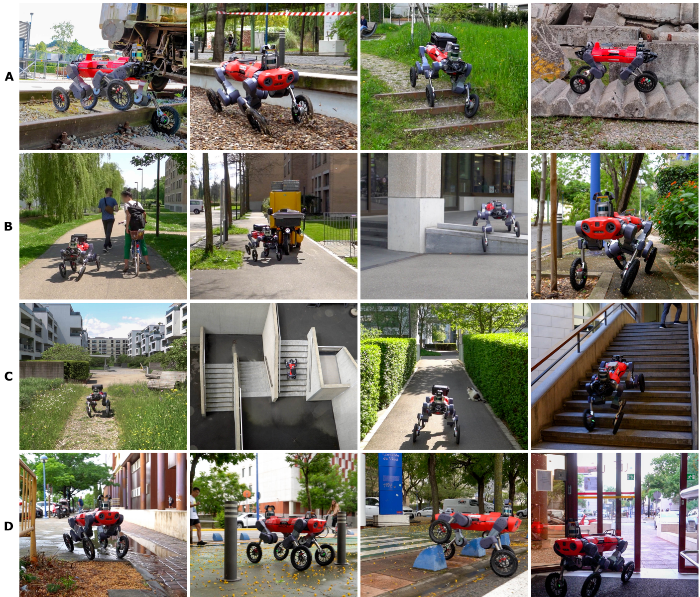
Fig. 1. Deployments in urban environments. Our control system for the wheeled-legged robot has undergone extensive validation in various indoor and outdoor locations. The experiments took place in Zurich, Switzerland and in Seville, Spain. (A) Locomotion challenges. (B) Navigation challenges; dynamic and static obstacles, complex terrains, and narrow space. (C) Locations in Zurich. (D) Locations in Seville.
