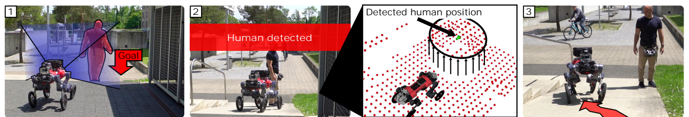
Fig. 5. Obstacle negotiation. (A) Our robot navigates around blocked routes by actively exploring the area and finding alternative paths. (B) Safe traversal of a narrow space. (C) Our robot exhibits two different ways to traverse the complex obstacle. (C, D) Our robot shows an asymmetric understanding of traversability, being able to traverse higher steps when going down. (D) We ensure safety around humans by incorporating additional human detection and overriding height scan values.
