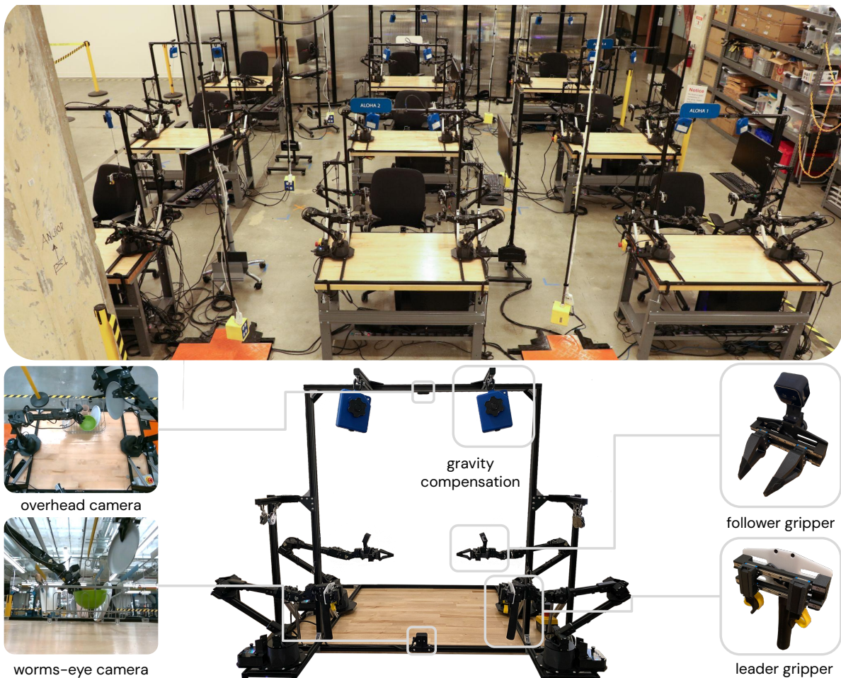
Figure 1 | ALOHA 2: An Enhanced Low-Cost Hardware for Bimanual Teleoperation . Top: The fleet of ALOHA 2 robots capable of collecting 1000s of demonstrations per day. Bottom: A detailed image of an ALOHA 2 workcell with gravity compensation, the redesigned leader and follower grippers, and images from the frame-mounted cameras.
