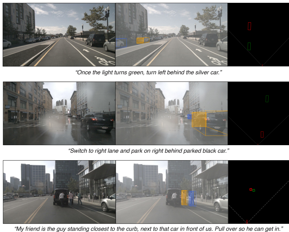
Fig. 13: Failure cases of Talk2Car images. The error mainly attributes to semantic mismatch. Each row has the original image (left), projected 3D box prediction and ground truth (middle), and BEV image (right). Blue box is the ground truth and Orange box is the prediction. In BEV images, Green box is the ground truth and red box is the prediction.
