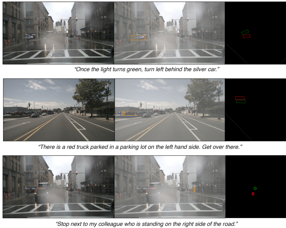
Fig. 12: Failure cases of Talk2Car images. The error mainly attributes to incorrect depth. Each row has the original image (left), projected 3D box prediction and ground truth (middle), and BEV image (right). Blue box is the ground truth and Orange box is the prediction. In BEV images, Green box is the ground truth and red box is the prediction.
