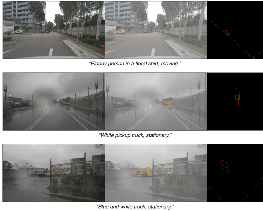
Fig. 10: Failure cases of DriveLM-Grounding images. The error mainly attributes to incorrect depth. Each row has the original image (left), projected 3D box prediction and ground truth (middle), and BEV image (right). Blue box is the ground truth and Orange box is the prediction. In BEV images, Green box is the ground truth and red box is the prediction.
