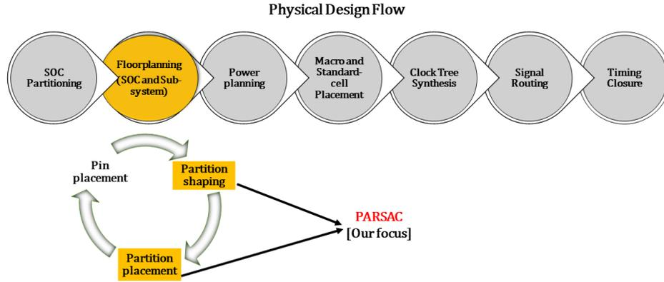
**Figure 1: The SoC and sub-system floorplanning task includes hierarchy-level partition shaping, partition placement and pin placement on the partition. Our work is applicable to both SoC and sub-system level partition placement and partition shaping.**
