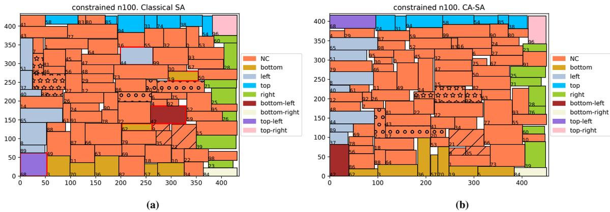
**Figure 6: (a) Sample floorplan from classical SA for the constrained n100 problem. There are five blocks that violate their boundary constraints. The violating blocks have a red outline. Blocks that are part of the same grouping constraint have the same fill pattern (circle, star, or cross-hatch patterns). (b) Sample floorplan from CA-SA for the same problem as a. All blocks satisfy the boundary constraints.**
