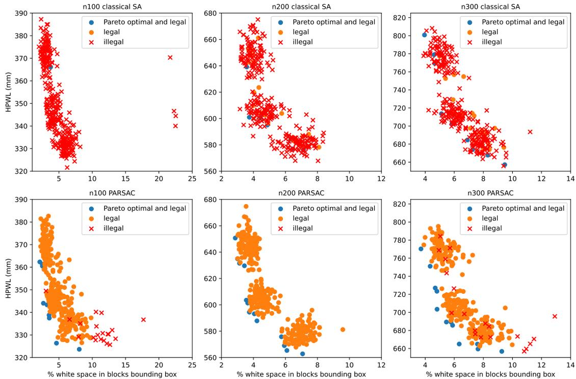
**Figure 7: The distribution of 336 solution points for the constrained n100, n200, and n300 problems for classical SA and PARSAC. We quantify the solution quality using the HPWL and the percentage of white-space in the block’s bounding box (the minimal box that contains all the blocks). The top rows shows the results for classical SA. Most of the floorplans are illegal. The bottom row shows the results for PARSAC which finds legal floorplans most of the time.**
