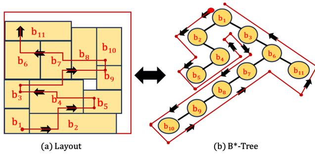
**Figure 2:** An example of a compacted floorplan (left) and the corresponding  $B^*$ -tree (right) representation. Given a compact layout, a tree representation can be obtained by traversing the blocks, starting from the lower-left module  $b_1$ . Likewise, given a  $B^*$ Tree, layout can be obtained by a DFS traversal, starting from the root node  $b_1$ .
