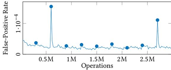
Figure 8: False-positive rate over time on dynamic workloads. Churning points are marked.
