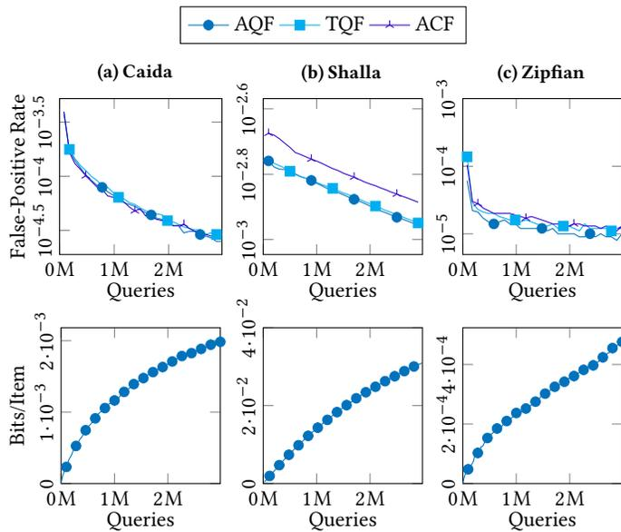
**Figure 7: False-positive rate (FPR) and additional space usage over time. FPR is on log scale. The adaptive filters are able to almost immediately reduce their FPR by up to 100× on a skewed workload. The ADAPTIVEQF is able to achieve a marginally lower or equivalent FPR at negligible space overhead.**
