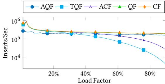
**Figure 5: System insert throughput as filter fills up.**
