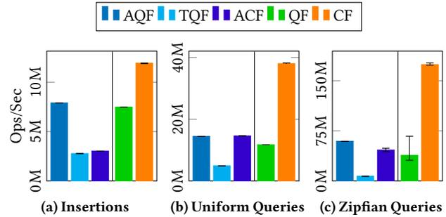
**Figure 3: Micro operation throughput of filters absent any system. Done by simulating a sequence of operations first, then returning and performing the same operations but on the filter alone. Adaptive filters are compared on the left, while nonadaptive filters are shown as reference on the right.**
