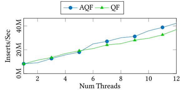
**Figure 4: Parallel insertion throughput.  $2^{26}$  slots in the filter.**
