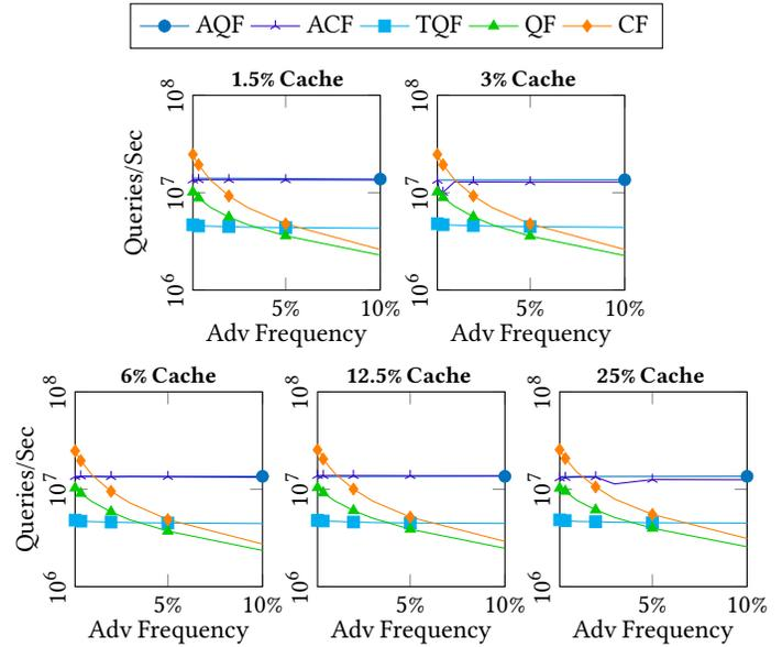
**Figure 6: Query throughput with varying cache size and frequency of adversarial queries. Each test included 100M warmup queries and 100M queries with an adversary.**
