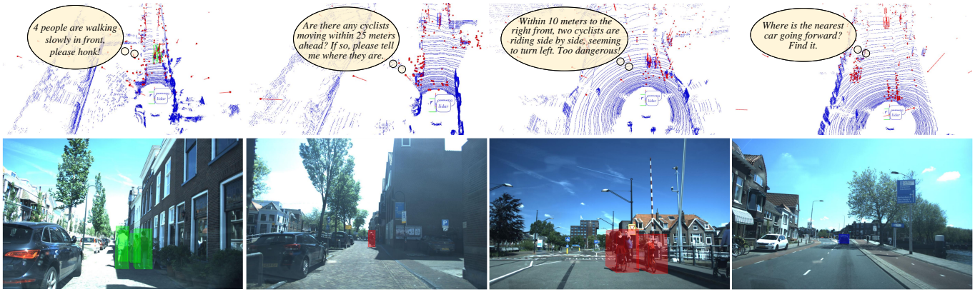
Fig. 1. Samples in Talk2Radar. The first and second row respectively presents referred objects by point cloud sensors (4D radar and LiDAR) and camera.
