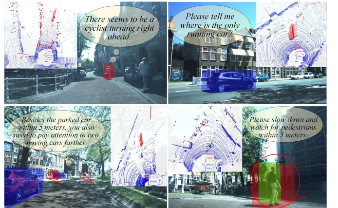
Fig. 5. Prediction by T-RadarNet. The first row presents correct cases while the second shows problematic cases (FN: False Negative, FP: False Positive).
