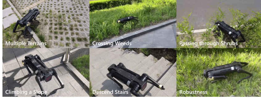
Figure 10: Real-world results for Aliengo robot with different joint failure in different terrains.
