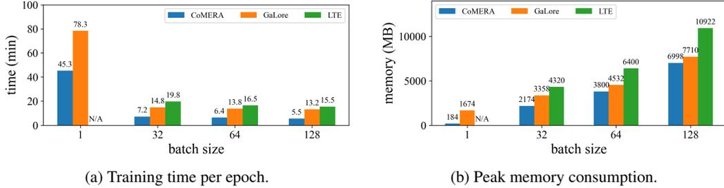
Figure 1: Training time and total memory cost of CoMERA, GaLore [37] and LTE [17] on a six-encoder transformer with varying batch sizes. The experiment is done on Nvidia RTX 3090 GPU.
