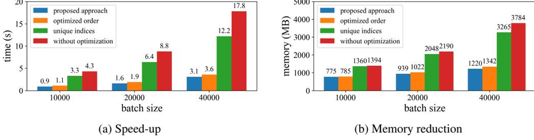
Figure 5: Performance of optimized TTM embedding table lookup. The labels *proposed approach*, *optimized order*, *unique indices*, *without optimization* represent the new method in 4.1, the method that only uses the unique order, the method that only uses the unique indices, and the method without optimization, respectively.
