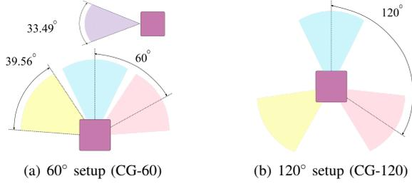
Fig. 2. Camera groups setup in our simulated datasets. FoV of the camera ( $39.56^\circ \times 33.49^\circ$ ) is calculated with the calibrated camera intrinsic. In this paper, we use three cameras to evaluate our algorithm.
