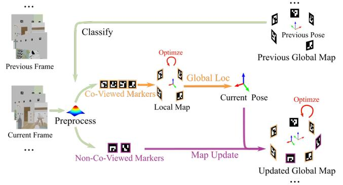
Fig. 3. The overview of our incremental marker-CG SfM framework is illustrated. The framework is divided into three parts: Preprocessing, Global Localization, and Incremental Map Update. Marker recognition and information confidence calculation are integrated in the preprocessing part. For clear statement, map initialization is not included in this overview.
