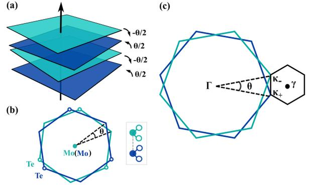
FIG. 1. Schematic diagram of ATML-MoTe<sub>2</sub>. (a) Schematic of AT4L-MoTe<sub>2</sub>, with the rotation directions of the 1st and 3rd layers (blue) opposite to those of the 2nd and 4th layers (green). (b) Top view of an AA-stacked AT4L-MoTe<sub>2</sub>. The inset shows a side view between adjacent layers. (c) Brillouin zones of the odd-layer (blue), the even-layer (green), and the moiré Brillouin zone (black).
