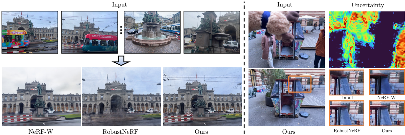
Figure 1. NeRF On-the-go . Given casually captured image sequences or videos in the wild as inputs, the goal of this paper is to train a NeRF for static scenes and effectively remove all dynamic elements in the scenes (cars, trams, pedestrians, etc), i.e. distractors. Unlike existing methods such as NeRF-W [27] and RobustNeRF [39], which produce imperfect results, our method leverages the predicted uncertainty maps to effectively remove those distractors. This results in high-fidelity novel view synthesis on challenging dynamic scenes.
