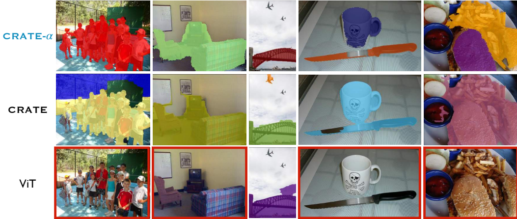
Figure 5: Visualization of segmentation on COCO val2017 [17] with MaskCut [38]. (Top row) Supervised CRATE- \alpha effectively identifies the main objects in the image. Compared with CRATE (Middle row), CRATE- \alpha achieves better segmentation performance in terms of boundary. (Bottom row) Supervised ViT fails to identify the main objects in most images. We mark failed image with \square .
