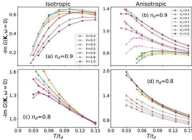
FIG. 4. Extrapolated antinodal zero-frequency  $-\text{Im}G(\mathbf{K}, \omega = 0)$  obtained from a linear extrapolation of the first two Matsubara frequencies at  $\mathbf{K} = (\pi, 0)$  (solid) and  $(0, \pi)$  (dashed).
