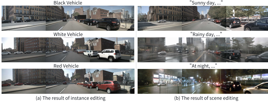
Figure 8: Visualization of instance and scene editing. (a) shows the instance-level control result, such as the appearance attributes of all vehicles. (b) shows the scene-level control result, including weather and time.
