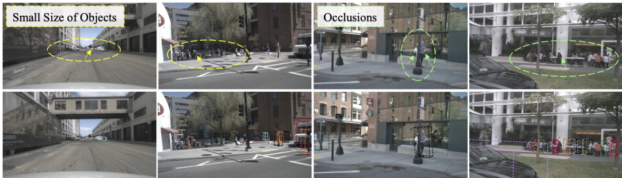
Fig. 1: The uncertainty issue in 3D multiple object tracking. The uncertainty issue refers to the models that do not provide accurate certainty estimates. In complex driving scenarios, the uncertainty issue arises from various factors, especially the occlusions and small size of target objects, which present significant challenges to achieving accurate tracking. The previous state-of-the-art end-to-end tracker, PF-Track [35], lacking uncertainty modeling, fails to track objects in certain complex scenarios.
