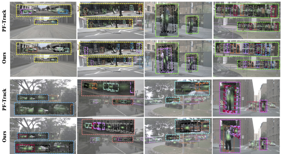
Fig. 8: More qualitative results on the nuScenes dataset. The tracking results on several challenging tracking scenarios with uncertainty, including the small size of the target objects and the occlusions. Moreover, we plot the attention scores of object queries, which indicate how strongly the model focuses on the target objects. A higher concentration of color represents a higher attention score and a stronger confidence in the corresponding object.
