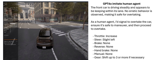
Figure 3: Example of GPT-4o imitating a human agent in the CARLA simulation. The LLM agent is attempting to overtake the car in front in a human-like manner.
