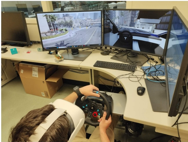
Figure 2: Simulation room with VR headset, steering controls, and monitors for real-time multimodal data collection and autonomous driving optimization.
