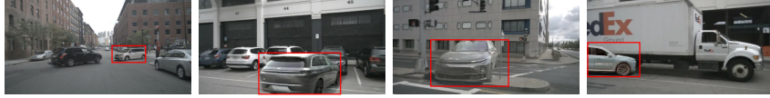
Figure 6: The simulated corner-case scenes. We use a red rectangle to highlight the simulated vehicles. These corner-case scenes show some vehicles have potential risks to traffic safety.
