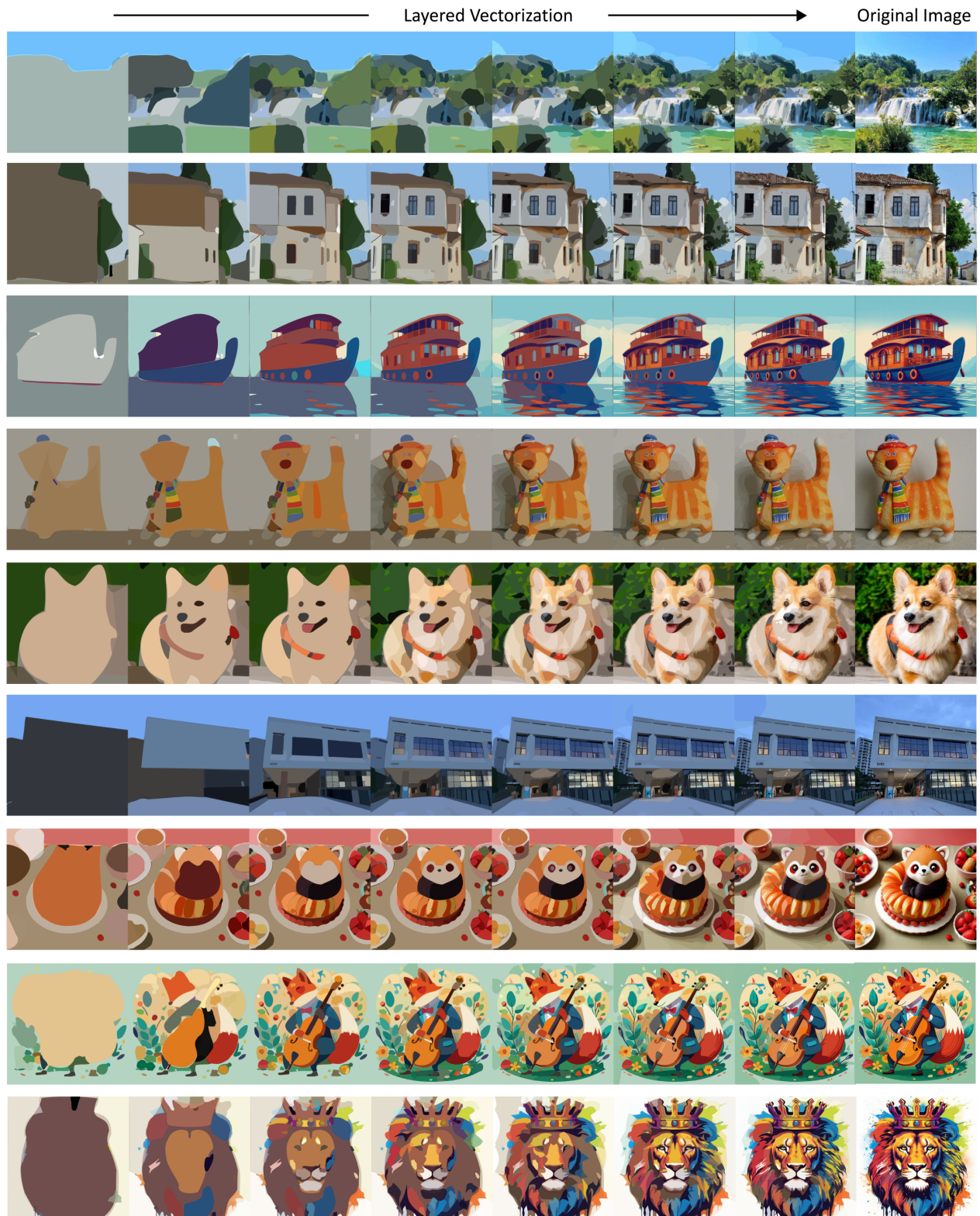
Fig. 10. Gallery of examples generated by our layered vectorization technique: given the input image on the right-most, our method progressively generates layers of vectors, transitioning from coarse to finely detailed representations. , Vol. 1, No. 1, Article . Publication date: June 2024.
